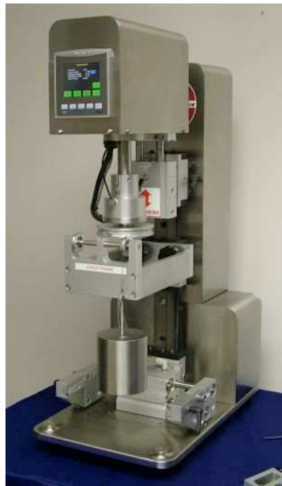
Figure 9: Calibration – Mechanical Setup for CCW calibration
