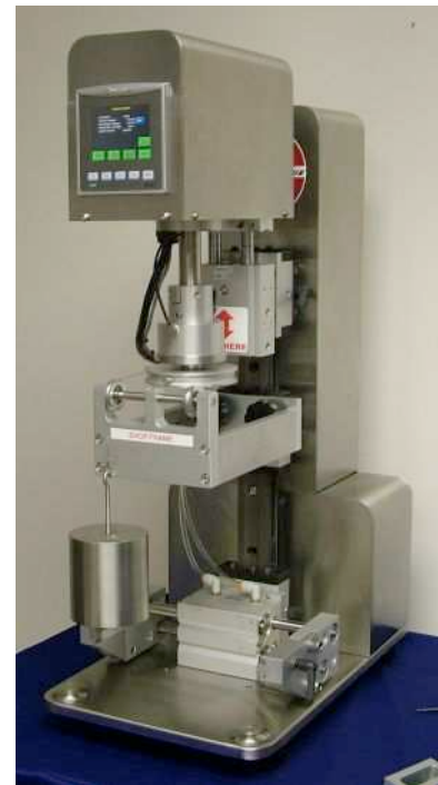
Figure 10: Calibration – Mechanical Setup for CW calibration
